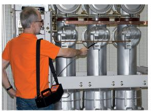
The measuring sensor extension (included in the scope of supply) allows measurements on measuring points difficult to access.
